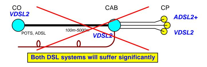
VDSL2/CO + VDSL2/CAB <u>cannot</u> coexist performance will degrade from both
