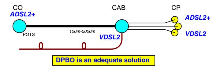
ADSL2/CO + VDSL2/CAB can coexist with adequate Downstream Power BackOff (DPBO)
