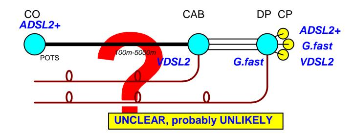
ADSL2/CO + VDSL2/CAB + G.fast/DP à coexistant? unclear if G.fast/DP should account for VDSL2/CAB
