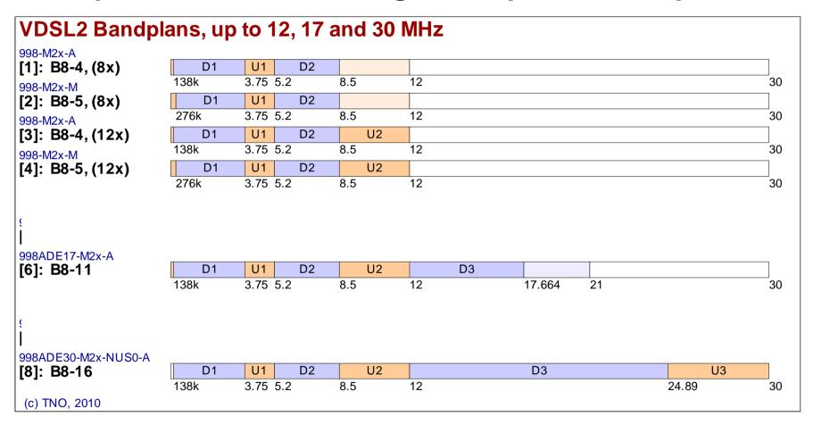
Option #2, select only bandplans that are spectrally compatible. Unbundling works well, just extending existing access rules
