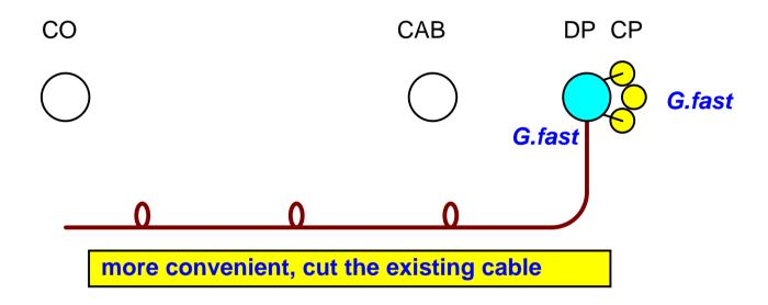
without any multi-node deployment one can cut the cable
