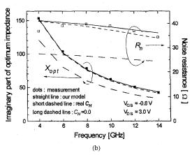
Fig. 5. (a) The minimum noise figure and the real part, and (b) the imaginary part of the optimum impedance and the noise resistance at  $V_{GS}=-0.8~{
