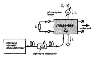
Fig. 2. Matched noise-tee configuration as an implementation of an electrical noise source with variable output level. The ratio between photo current  $I_d$  and spectral current density  $(\sqrt{S_{ie}})$  of the excess-noise is insensitive to optical power variations.
