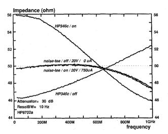
Fig. 4. Output impedance measurements on a matched noise-tee configuration (Fig. 2) and a conventional noise source (HP346c). The p-i-n photodiode is biased at a constant voltage of 20 V. The dc photo current at maximum illumination level is 750  $\mu A$ .
