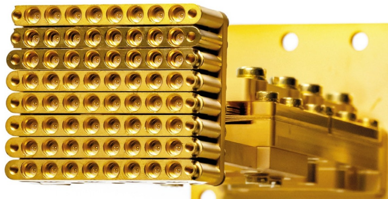
Figure 7.3. An example room-temperature node with 64 coaxial connections
