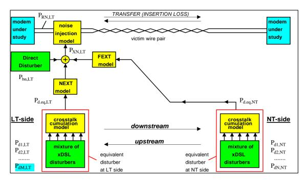
Figure 6: Flow diagram to evaluate the crosstalk probability limits for two-node topologies, at the LT side (for evaluating upstream performance)
