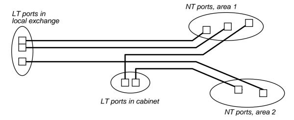
Figure 3: Example of the wiring in a multi-node topology.
