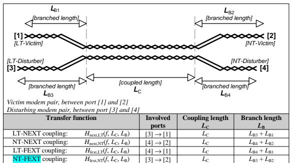
Figure 2: Example of the lengths that are to be used for evaluating branched normalized NEXT and FEXT
