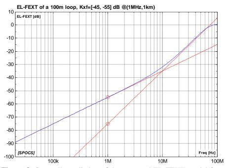
**Figure 3.** Crosstalk prediction of the proposed EL-FEXT model for a 100m loop, using the same parameter values as in figure 2. Since the vertical offset of both asymptotes scale differently with the cable length, the break frequency in this figure (10 MHz) is different from its value in the previous figure (3 MHz).
