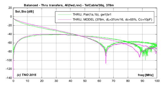
**Figure 1** Match between a sample cable measurement and the full multi-port model proposed in [1]. Both transmission and FEXT are well predicted by the model, and this even applies to the dip in transmission near 64 MHz.
