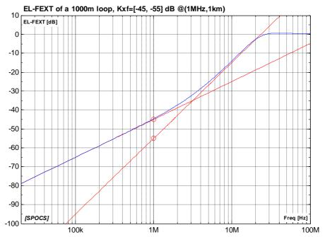
**Figure 2.** Crosstalk prediction of the proposed EL-FEXT model, for a 1km loop, when the model is characterized as  $K_{xf1}$ = -45 dB and  $K_{xf2}$ = -55 dB, both specified at 1 MHz and 1km. The asymptotes are crossing at 1 MHz the values of  $K_{xf1}$  and  $K_{xf2}$  since it is a 1 km loop.
