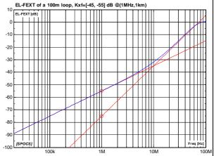
**Figure** [\*]b. Crosstalk prediction of the EL-FEXT model for a 100m loop, using the same parameter values as in figure [\*]a. Since the vertical offset of both asymptotes scale differently with the cable length, the break frequency in this figure (10 MHz) is different from its value in the previous figure (3 MHz).
